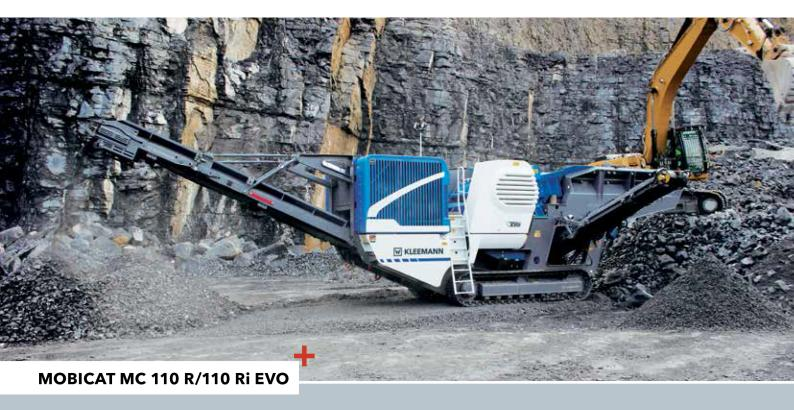
The MC 110 R EVO is characterised by an impressive output in its class and by the vibrating feeder with integrated slotted grate. The plant is used as a primary crusher in natural stone and in demolition and recycling companies. Thanks to its low weight, it is easy to transport and flexible in operation.
